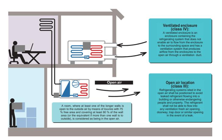
**EN 378, Part 3, Clause 4, defines requirements and directions for location of refrigerating equipment**. There are greater limitations for equipment located in occupied spaces than for a machinery room, open air or ventilated enclosure located within an occupied space.
